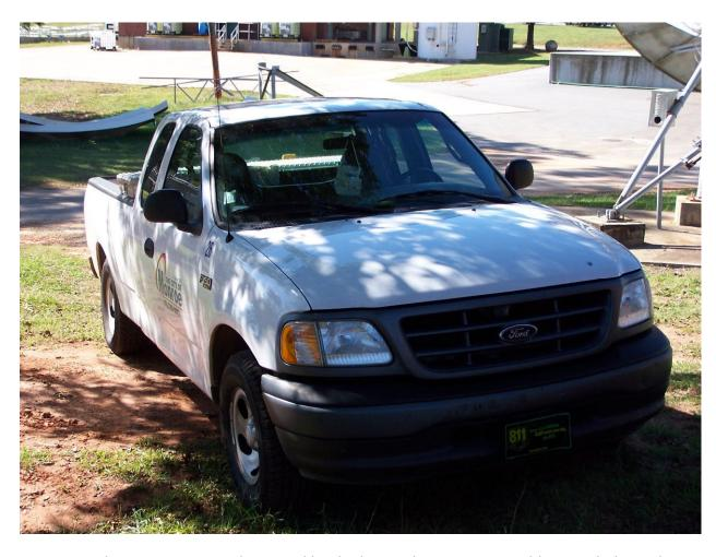
2002 Ford F150 185,000+ miles. Used by the locate department. Problems include intake, brake system, engine block, and electronics. Replace with Ford F150 budget price \$25,000.00
